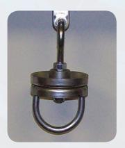
Earl Monroe, PACLINE's fabricating supervisor and Robert developed a simple custom hook design that would handle all types of cylinders. This was all tested in PACLINE's conveyor testing facility.
