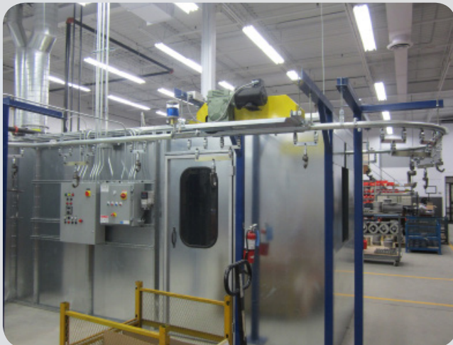
PACLINE motor and lubricator are wired to the control panel.
