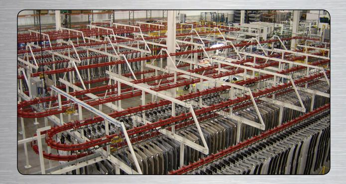
This PACLINE power and free conveyor supports an ILVS (In Line Vehicle Sequencing) process. The conveyor facilitates sequencing and storage of automotive interior roof panels, buffering 500 parts (25 lbs. each) on 7 inch centers. The track allows for close-pack accumulation in the straight section, then singulates around each 180 degree curve.
