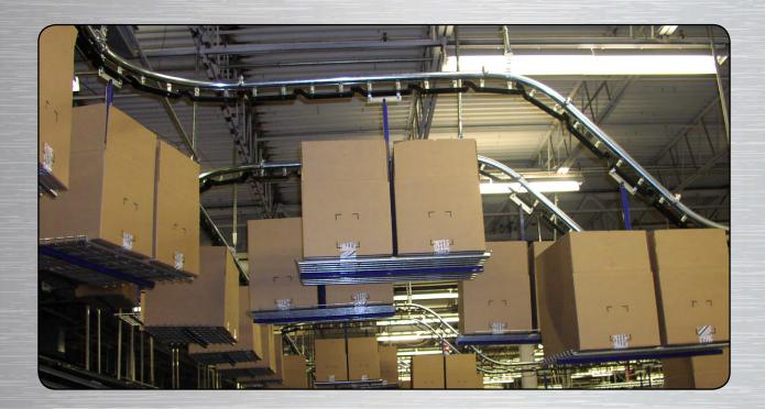
In this facility the PAC-LINE™ overhead conveyor system is being used to automate the delivery of empty cartons. Two conveyor loops (810 ft. and 580 ft.) are installed above a roller conveyor in this large distribution center to service the 'put to light' system for retail clothing store replenishment.
