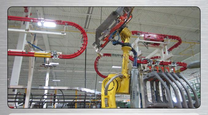
This PACLINE Power and Free conveyor is used to buffer parts between welding operations. The conveyor allows parts to be accumulated and drawn from on a first-in-first-out basis and to cool down while buffering. The flexibility of our power and free conveyor allows for empty carriers to return over the full carriers below.
