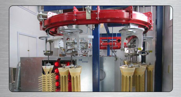
The PAC-MAX™ enclosed track overhead conveyor is used to transport investment casting slurry molds through a curing line. Here, custom rotators carry 150 lb. parts through a specialized dehumidifier booth. The customer integrated this system with a robotic part handler for transferring molds between processes.
