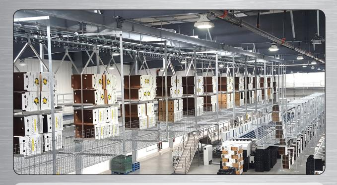
This citrus fruit packing operation uses the PAC-LINE™ enclosed track overhead conveyor with multi-level carriers (8 boxes per carrier) to deliver empty cartons to fruit packers on the floor. Cartons are transferred from the box-building area up into the ceiling area to keep the floor area free for the high speed sorting equipment.
