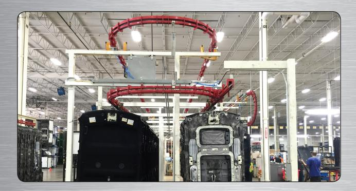
Automotive headliners can be difficult to handle, however the PACLINE power and free overhead conveyor provided an excellent buffer system for this In-line Vehicle Sequencing system. The accumulated headliners are moved sequentially, allowing just enough time between car assembly plant broadcast and headliner production.
