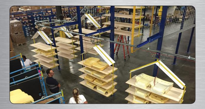
Foam seat cushions for automobiles are loaded on these custom carriers for transport in this assembly operation. The PAC-LINE™ conveyor can handle very sharp inclines to move loaded carriers up off the floor level. Transportation is timed so that the newly manufactured seat cushions complete the curing process by the time they reach the unload area.
