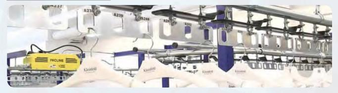
The PAC-LINE™ enclosed track overhead conveyor has proven to be the ideal solution for the garment handling system at KLEINFELD.The final design included two independent conveyor loops, each with their own RETRIEVER™ control system.
