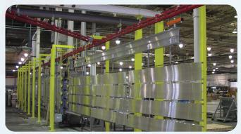
The first step in the process is loading the conveyor. To minimize handling of panels, the loading of the conveyor was positioned right next to the punch press where mating holes are punched into the sign panels (holes are used for final assembly). Once the holes are punched, an operator loads the panels onto the carriers of the Power and Free conveyor system. Each carrier was designed to hold multiple panels for maximum efficiency.
