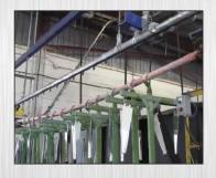
All conveyors are designed to withstand the harsh chemicals and high oven temperatures involved in the powder coat and e-coating processes.
