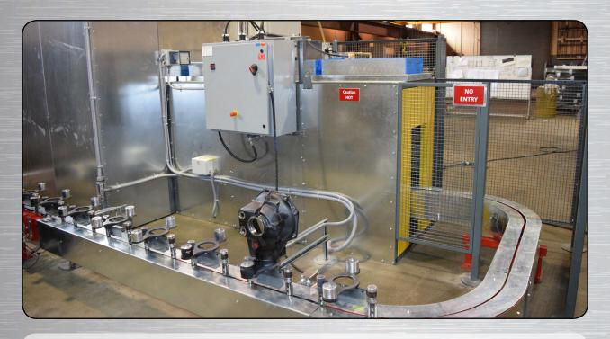
This PACLINE Power and Free conveyor is inverted and floor mounted for a robotic wet spray system for precision painting machined automotive parts. The power and free, asynchronous system allows the customer to buffer parts at load and unload while other parts continue through the painting and curing stages.
