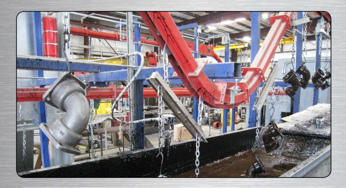
The heavy duty PAC-MAX<sup>™</sup> conveyor is handling 80 lb. parts through a dip line painting process. This system has the capability of handling parts up to 400 lbs. per load bar. The tight radius vertical curves of the conveyor track help minimize the size of the dip tank and allows for a very compact overall system.
