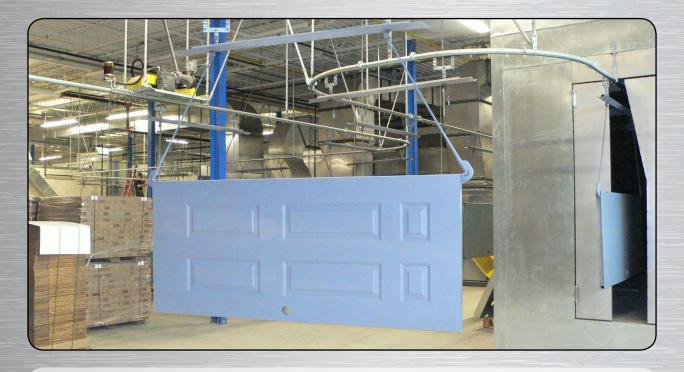
This paint finishing line uses the PAC-LINE™ enclosed track conveyor to transport metal doors through a wet spray booth and curing oven. The conveyor track is installed at the ceiling to leave the floor area clear. Tall hanging items such as these doors can be hung vertically or horizontally depending on the process and size of the ancillary equipment.
