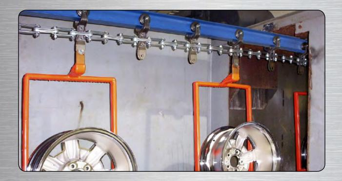
This PAC-BEAM™ conveyor system with heavy duty chain and trolleys transports automotive rims through a chemical wash process. Custom carriers are rubber coated to prevent corrosion and I-Beam track is stainless steel in sections that pass through the washer.
