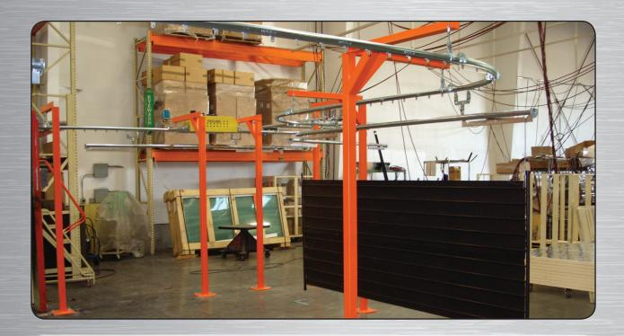
This PAC-LINE™ conveyor system was used to carry solar panels of varying lengths through an automated paint booth. The system included a unique "bar trolley" carrier that allowed the long panels to move easily around the 3'-0" radius horizontal curves. The "bar trolley" carrier also included hooking points at various spreads that could be selected by the operator.
