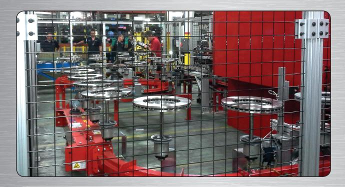
Painting these quality automotive brake rotors with automated spray guns required that the parts be rotated at a highly consistent rate. The Pacline enclosed track PAC-MAX™ conveyor was selected as it provided excellent stability when floor mounted, in the slot sideways position. Having the parts move above the track also ensured a very clean paint finish.
