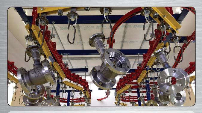
The PACLINE power and free conveyor is used in this unique painting process. Steel valves are spray painted and cured within the same room. The power and free system allows for the drive unit to be located outside of the paint/oven room and therefore protected from the high temperatures during curing. Parts are hung by rotators to ensure even paint coverage.
