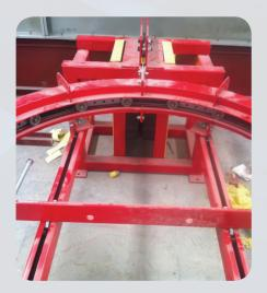
In addition, the take-up unit for this system was a gravity powered counterbalance design. This take-up provided uniform tension with NO power requirements and the capabilities to add or reduce weight to suit the application.
