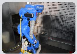
Incorporating a robotic spray paint system had a number of advantages. First, it required minimal space to operate which was particularly important for this installation. And secondly, since the parts did not require overall painting but rather spot painting, the robot could deliver this in a much more precise manner compared to hand spraying. With very little paint overspray, the system was kept clean and reduced wasted paint.
